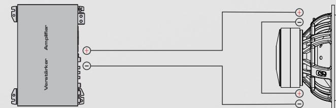
2 Subwoofer Parallel/Serial wiring: 2 Ohm
